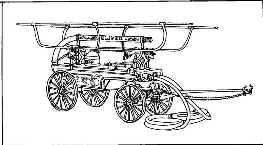
The "double stream piano deck fire engine" shown in this drawing takes its name from the fact that its body resembles the rectangular pianos that were in vogue in 1895, when the style was first introduced. Eighteen men, nine to a side, worked 15-foot pump levers to throw twin streams of water,  $\frac{3}{8}$ " in diameter, for distances of over 100 feet.
